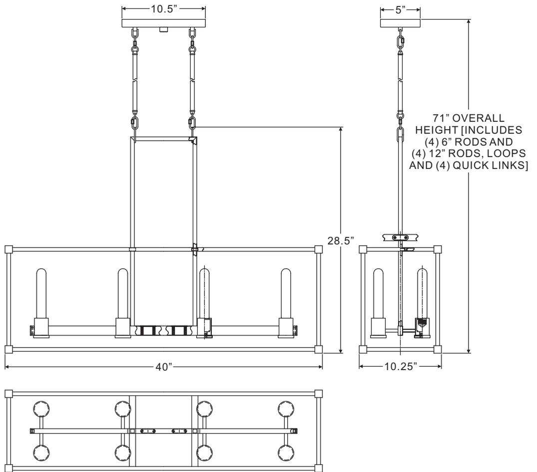
71" OVERALL HEIGHT [INCLUDES (4) 6" RODS AND (4) 12" RODS, LOOPS AND (4) QUICK LINKS]
