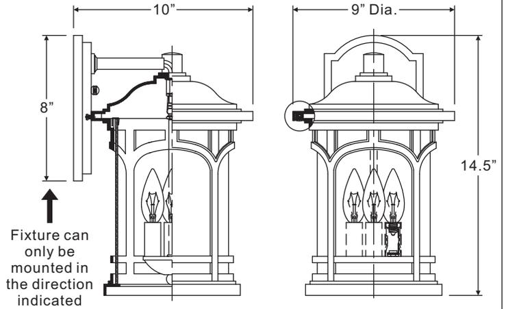
Fixture can only be mounted in the direction indicated
